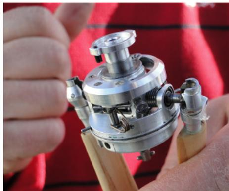
**Propeller hub of rubber powered model**
