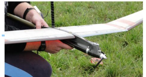
**Nose of a power model (class F1C) with fully integrated motor**
